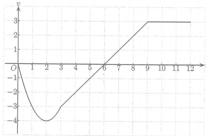
i) Given that the velocity  $v = t^2 - 4t$  for  $0 \leq t \leq 3$ , find the displacement of the particle during this time.
